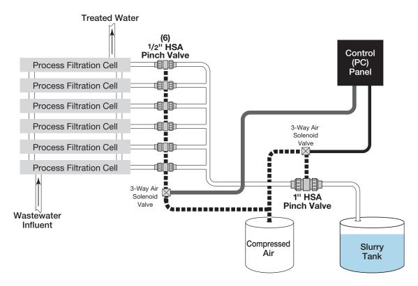
Prior to wastewater being released into the system, the HSA Pinch Valve is used to introduce the slurry mix into each process cell. Once the cells are filled, the Pinch Valves are closed and the wastewater is released onto the system where the water is filtered and purified. Both a Ball Valve and a Diaphragm Valve were
