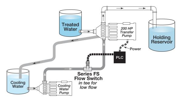
Large pumps used in municipalities for water and waste water transfer are quite expensive, usually in the tens of thousands of dollars. To prevent premature bearing failure, cooling water is used in the pump head where the bearings are located. The cooling water typically flows at 0.5 gpm.
