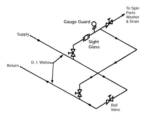
Following the manufacturing of chips, they are placed into a Spin Parts Washer where D. I. water is used to clean the chips under pressure and spraying. Chips are then spun air-dried, and used for final assembly. Sight Glasses are utilized to permit watching the fluid for visual color change in the D. I. water (algae-green). The Gauge Guard is used to confirm a constant pressure during the wash cycle. D. I. water is sent down drain after each use.
