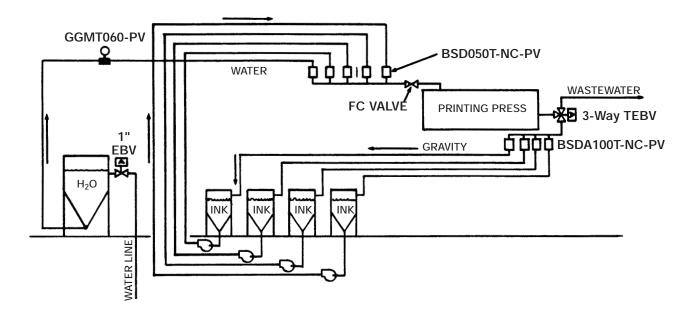
Water-based printing inks are corrosive and tend to adhere to and build-up on valve seal surfaces causing leakage. The Series BSD Diaphragm Valves (pressure supply valve) were chosen for their non-adhering PTFE diaphragms and automation of ink delivery that was previously fed by manual valves. Once the presses stop another BSD opens, allowing water to flush the line. The 3-Way TEBV True Blue
