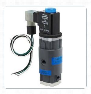
Diverter or "sampling" valves with no metal parts in wetted area. Design features a non-sticking shaft with an upper and lower diaphragm separating the liquid from opposing springs, plus secondary seals with Fail Dry safety vents. Suitable for all solutions. Series THP is not specifically designed for vacuum service; consult factory if needed.
