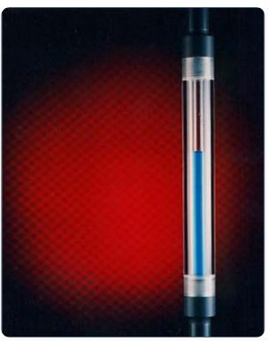
Although these flow indicators have no specific inlet or outlet, care should be exercised when installing such units that have streamers for fluttering devices. They must be installed in such a manner that the fluid flow will force the streamers into the indicator's viewing area.
