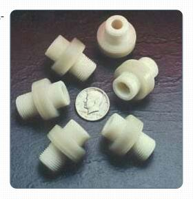
Series GGMU — Ultra-Pure Gauge Guards with Spigot End Connectors — Zero dead-leg design with EPDM or Viton sleeve; ultrapure connection via natural polypro, Kynar PVDF, or PVC. Pipe sizes 1/2", 3/4", 1", 1-1/2", and 2". Rated full vacuum (Gauge Guard MUST be solidly filled to function properly with process vacuum) through 200 PSI.
