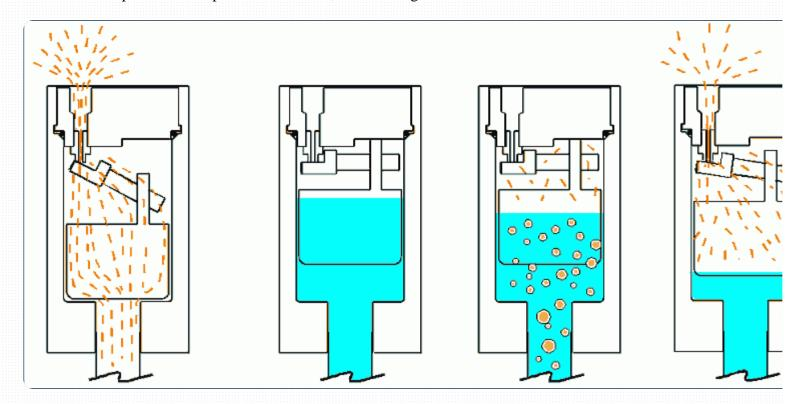
The valve has a very small orifice and is designed for trace amounts of gas. To expel large volumes of air such as at system start-up, see Series ARV . If your application requires expulsion of a large amount of air, as well as periodic venting of smaller amounts, you may require both the Series ARV and Series DGV.
